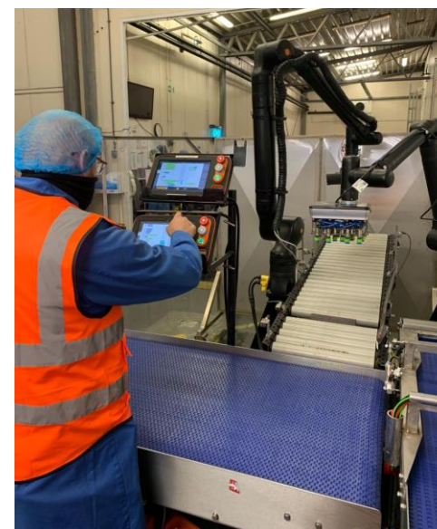
C-Tech Project – Moveable and Collaborative Robotic End-of-Line Packing ( industry first )
