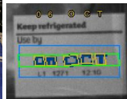
C-Tech Project – Machine vision system identifying, locating and checking product date code in real-time
